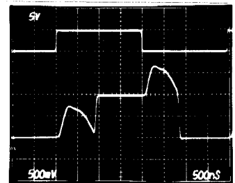
MUX-24 SMALL-SIGNAL SWITCHING WITH 2μs SAMPLE TIME
