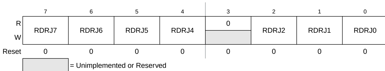
Figure 23-59. Port J Reduced Drive Register (RDRJ)
