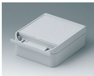
C6013161 SMART-BOX WIDTH 5.118" ASA+PC-FR (UL 94 V-0) light gray RAL 7035 6.30"x5.12"x2.36" IP 66
