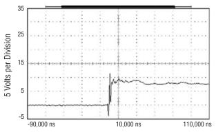
ESD Test Pulse - 25 kilovolt, 1/30 ns (waveshape)
