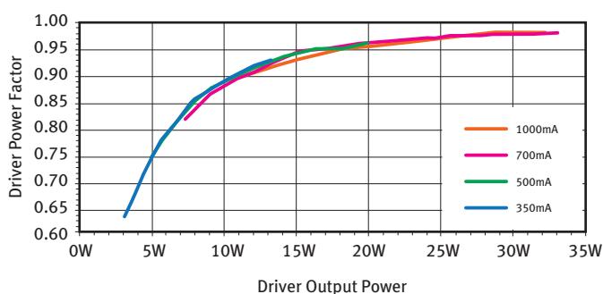
Driver Power Factor Characteristic at 230V Input
