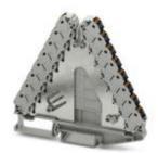
Potential distributors, Nom. voltage: 250 V, Nominal current: 17.5 A, Cross section: 0.14 mm² - 2.5 mm², AWG: 14 - 26, Connection type: Push-in connection, Width: 8.3 mm, Length: 100 mm, Color: gray, Assembly: NS 35/7,5, NS 35/15
