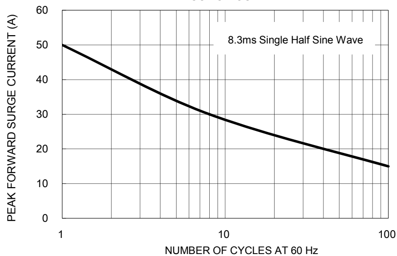
FIG. 3 MAXIMUM NON-REPETITIVE PEAK FORWARD SURGE CURRENT
