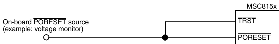
Figure 35. Reset Connection in Functional Application
