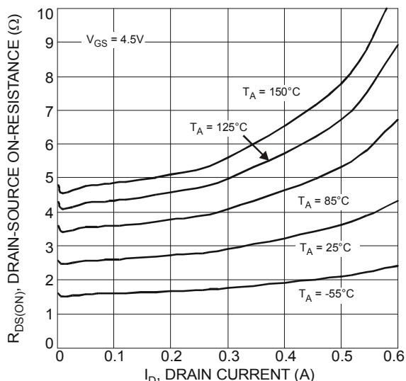
Figure 5 Typical On-Resistance vs.
