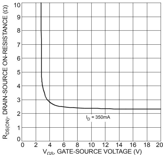
Figure 4 Typical Drain-Source On-Resistance
