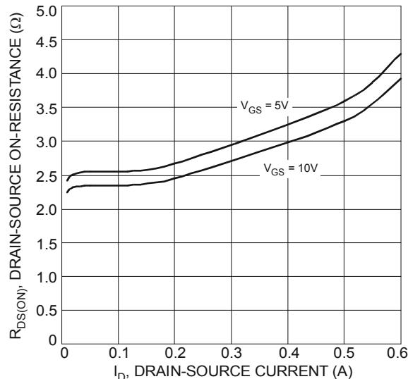
Figure 3 Typical On-Resistance vs.
