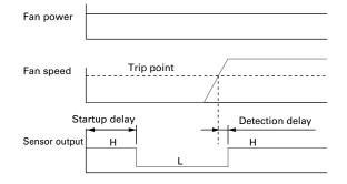
Startup delay: 18±3 s Detection delay: 3 s MAX. Trip point: 1,700 min<sup>-1</sup>
