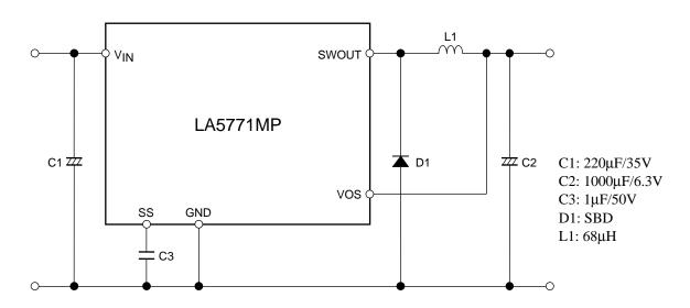
Notes: C3 is for the soft start function. Delete C3 and keep the SS pin open when the soft function is not necessary.
