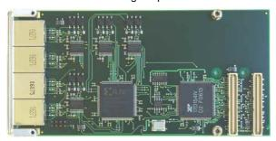
Each RS232 channel supports RxD, TxD, RTS, CTS and GND. RS422 and RS485 full duplex support a four wire interface (RX+, RX-, TX+, TX-) plus ground (GND). RS485 half duplex supports a two wire interface (DX+, DX-) plus ground (GND).
