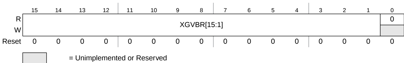
Figure 6-5. XGATE Vector Base Address Register (XGVBR)
