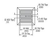
For Sculptured: Note maximum space available for 1 or 2 line legends. These dimensions must be considered when choosing font style and size for round printable area of cap lens, diffuser, insert or film insert.
