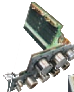
FLEX CIRCUITRY WITH RECTANGULAR CONNECTORS
