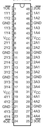
The 74ACT16244 is packaged in TI's shrink small-outline package, which provides twice the I/O pin count and functionality of standard small-outline packages in the same printed-circuit-board area.
