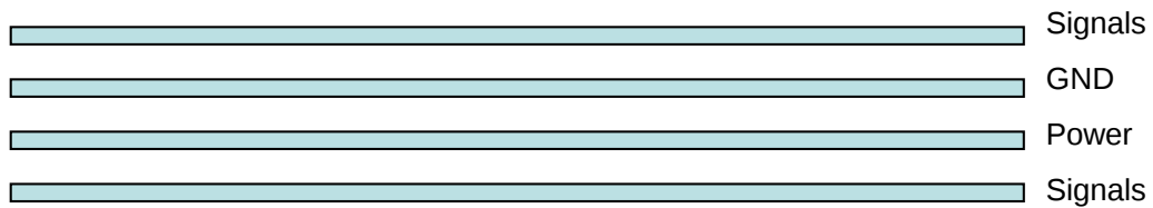
Figure 18: Typical 4-layer PCB construction
