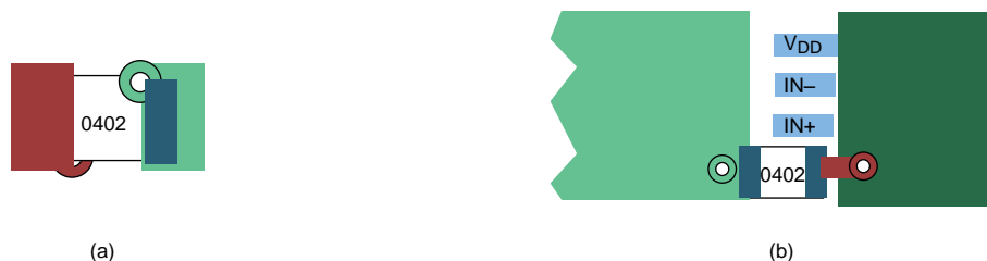
Figure 27. Typical Decoupling Capacitor Layouts
