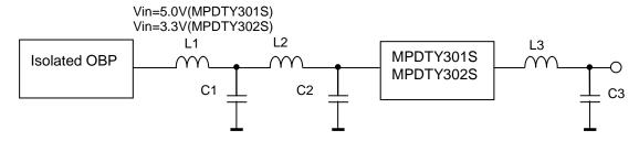
When the isolated OBP in the above Fig is MPD6D128S, or some OBP that has less output inductance than 1.6  $\mu$  H and much output capacitance than 200  $\mu$  F.
