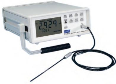
The Model 6010 Hall-effect gaussmeter represents the latest innovations and state-of-the-art designs from the world leader in magnetic measuring equipment. F.W. Bell's exclusive *Dynamic Probe Correction* feature, along with temperature compensation, allows measurements up to 300 kG with a basic accuracy of 0.25%.
