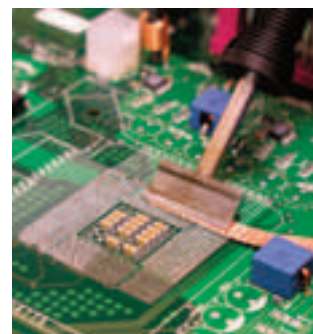
BGA pad cleaning with SMTC blade tip cartridge. See full range on page 20.
