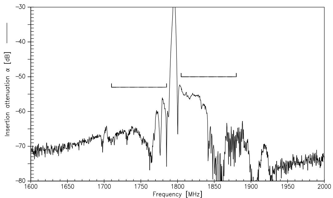
Frequency Response TX-RX (differential mode, wideband)
