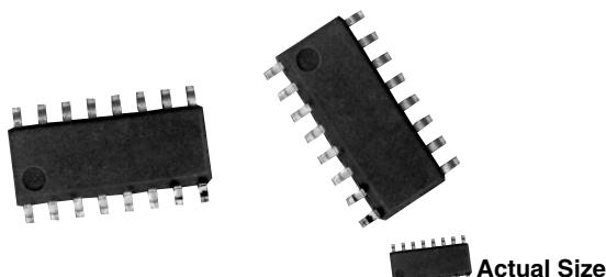
The NOMC series features a standard 14 pins and 16 pins narrow body (0.150") small outline surface mount style. It can accommodate resistor networks to your particular application requirements. The networks can be constructed with passivated nichrome (standard), or tantalum nitride <sup>(1)</sup> resistor films to optimize performance.
