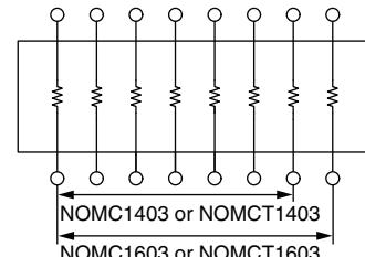
The 01 circuit provides a choice of 13 or 15 equal value resistors each connected between a common lead (14 or 16). Custom schematics available.
