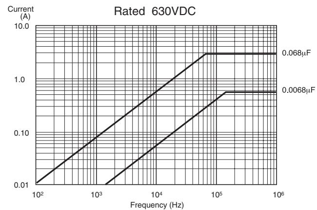
**Typical Characteristic Curves** Remarks : Typical curves are as shown below.(Slightly different depending on individual rating.)
