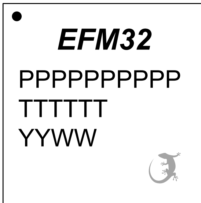
Figure 8.3. BGA120 Package Marking
