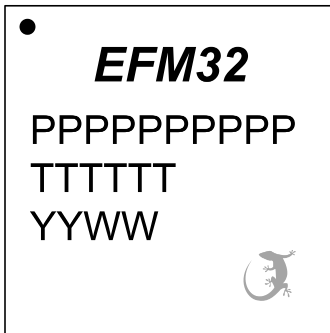
Figure 7.3. BGA152 Package Marking
