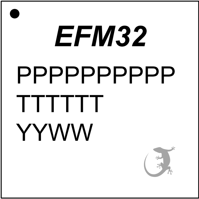
Figure 11.3. TQFP64 Package Marking
