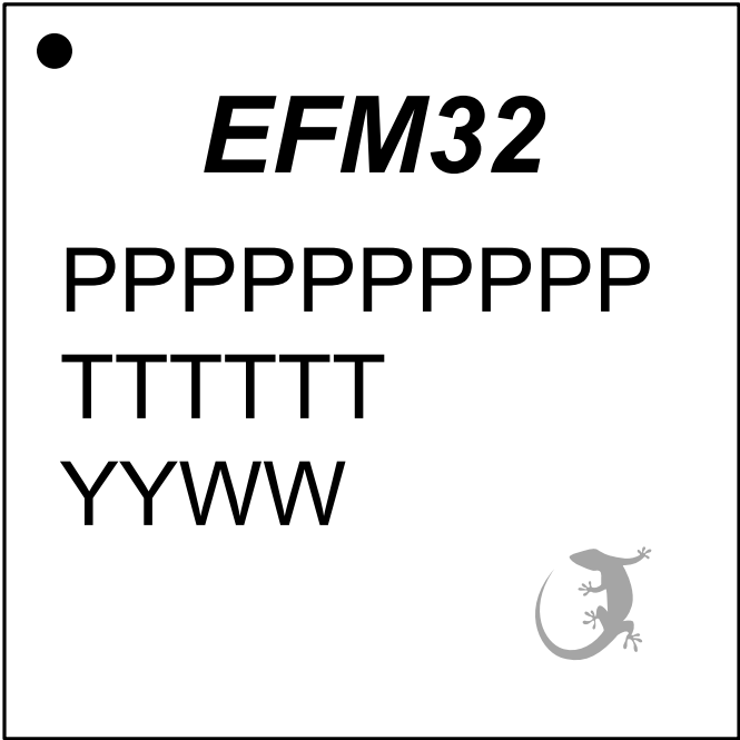
Figure 10.3. TQFP100 Package Marking
