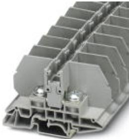
Feed-through terminal block with bolt connection method, cross section: 2.5 - 35 mm<sup>2</sup>, AWG: 12 - 2, width 17 mm, color: gray
