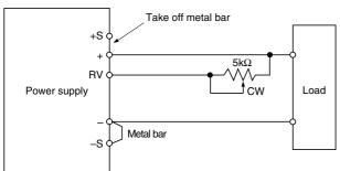
Remove a bar between +S and + terminals.
