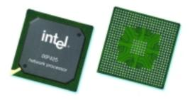
With their Development Platform, a choice of operating systems, and a broad range of development tools, the Intel IXP425 network processors provide a complete development environment for faster time-to-market. This network processor family offers the choice of multiple clock speeds at 266, 400, and 533 MHz, with both Commercial (0° to 70° C) and Extended (-40° to 85° C) temperature options.
