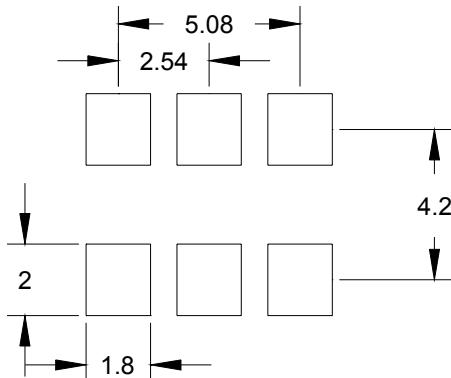
Note: XPRESSO LVPECL XOs are designed to fit on Industry standard, 6 pad, layouts.
