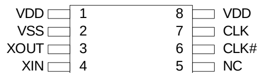
Figure 1. Pin Diagram - 8-Pin TSSOP
