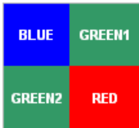
Figure 3. Color Filter Arrangement on the Pixels
