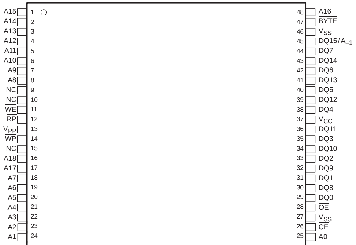
TMS28F800Axy 48-PIN TSOP (DCD) (TOP VIEW)
