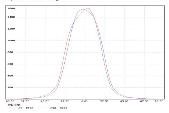
Luminaire: Ledil Oy CA13100\_TINA3-W (Luxeon RE-ES 92lm @ 250mA) Efficiency=91% Lamps: 1 x Luxeon RE-ES 92lm @ 250mA
