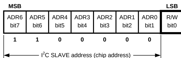
Figure 36. I 2 C Chip Address
