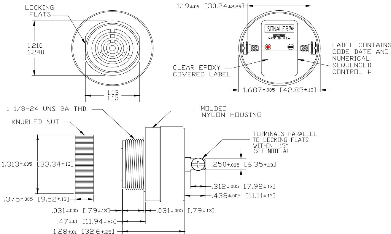
NOTE A: TERMINALS-.032 BRASS TIN PLATED, TAPPED FOR #6-32 SCREW. TWO #6-32 NICKEL PLATED BRASS SCREWS INCLUDED. WILL ACCEPT 1/4" QUICK CONNECT.
