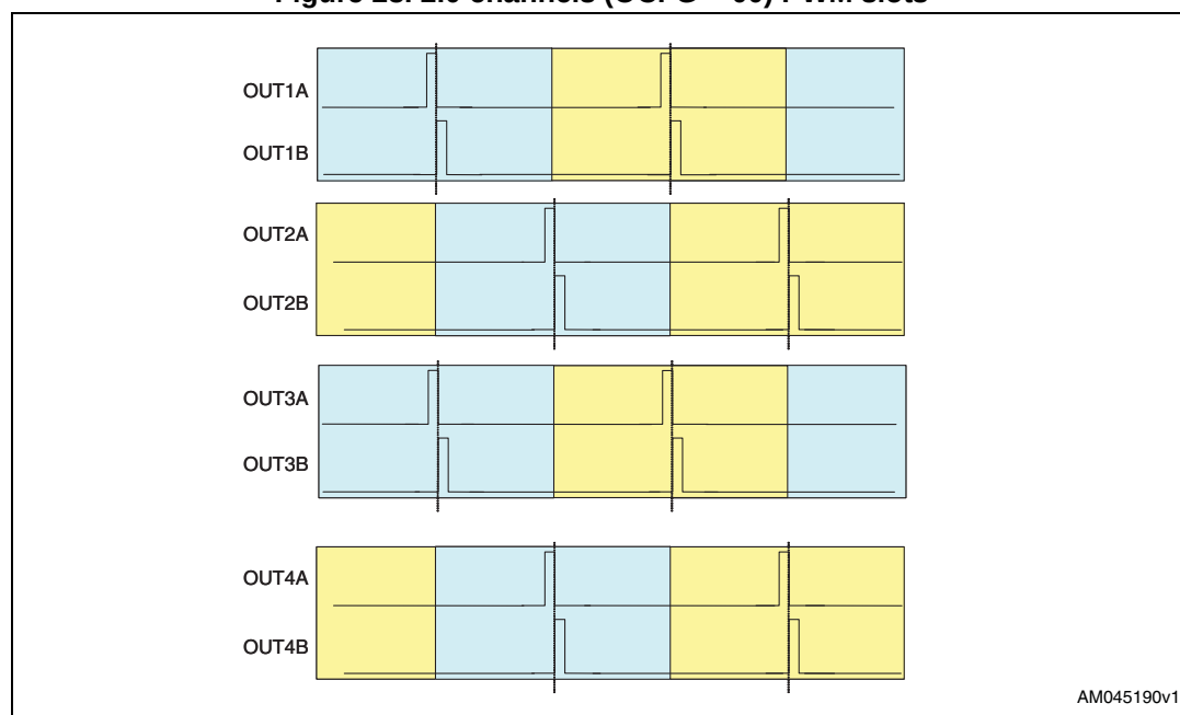
Figure 28. 2.0 channels (OCFG = 00) PWM slots
