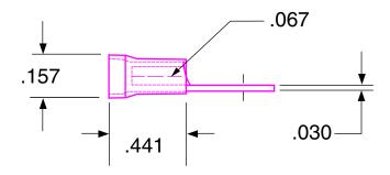
Max Electric Currrent: 22-16 AWG : 19 Amp Max Electric Rating: 75° C / 600 V Max
