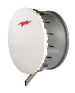
1.8 m | 6 ft High Performance Parabolic Shielded Antenna, single-polarized, 4.400–5.000 GHz, CPR187G, gray antenna, enhanced white radome with flash, standard pack—one-piece reflector
