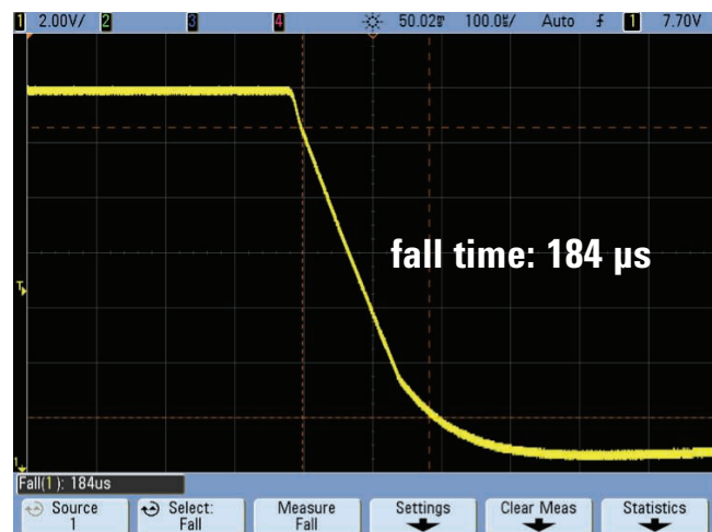
Figure 5. Interrupt pulse fall time measurement of < 200 \mu\text{s}
