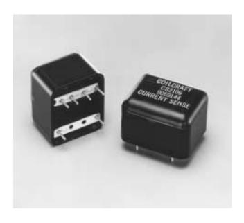
These Coilcraft current sense transformers are intended for use in measuring 50/60 Hz line currents from 0.5 to 20 Amperes RMS. Typical application as shown below yields a standard output of 0.1 Volt per Ampere. The sensitivity may be changed easily by simply adjusting the value of the sense resistor. These parts also can be used to measure 400 Hz line currents.
