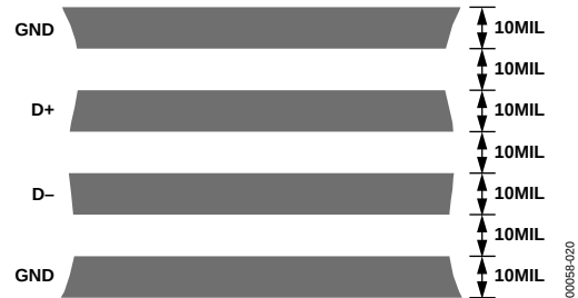
Figure 20. Arrangement of Signal Tracks
