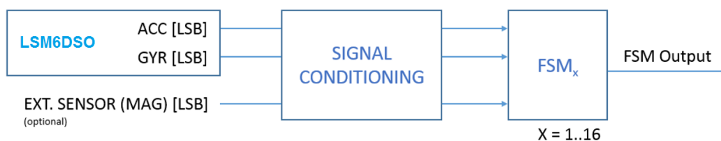
Figure 2. State machine in the LSM6DSO
