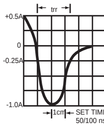
FIG. 5 - TEST CIRCUIT DIAGRAM AND REVERSE RECOVERY TIME CHARACTERISTIC
