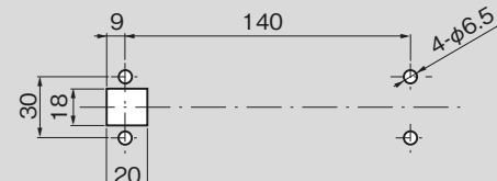
[A-869-2] パネル穴明け寸法 Panel drilling dimensions
