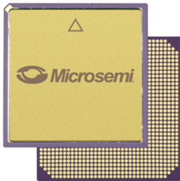
CB1657/CG1657/LG1657 RT4G075, RT4G150 b.s. 1.693x1.693" (43x43mm) h. CBGA - 156 mils (3.97mm) h. CCGA - 213 mils (5.42mm) h. CLGA - 126 mils (3.21mm) p. 39 mils (1.00mm)
