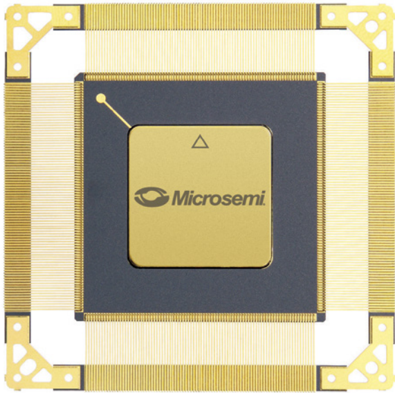
CQ352 b.s. 1.890x1.890" (48.00x48.00 mm) h. 105 mils (2.67 mm) p. 20 mils (0.50 mm)
