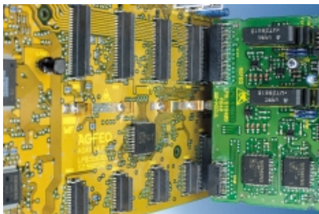
Male and Female connectors in ISDN equipment
