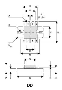
SOURCE (COMMON) PIN 2 PIN 1 DRAIN 1 SOURCE (COMMON) PIN 3 DRAIN 2 PIN 4 PIN 5 SOURCE (COMMON) PIN 6 GATE 2
