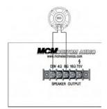
If multiple speakers are connected, they may be connected in series, as shown in the adjacent illustration. In this case, you simply add the impedance of each speaker. Two  $8\Omega$  speakers connected in series create a 16 load. This arrangement is normally only practical when four or fewer speakers are used.
