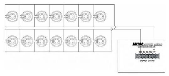
Typically, speakers having attached 70V transformers will have multiple wattage taps available for connection. For example, the very popular MCM Custom Audio ceiling speaker, Model #555-9018, includes taps for 0.325W, 0.625W, 1.25W, 2.5W, 5W and 10W. The popular outdoor speaker Model #80-492 includes a rotary selector for selection of 5W, 10W, 20W and 30W.
