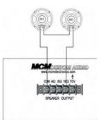
The adjacent illustration demonstrates a parallel connection. In this case all speakers must be the same impedance. You divide the impedance of one speaker by the total number of speakers connected. Two  $8\Omega$  speakers connected in parallel creates a  $4\Omega$  load. This arrangement is normally only practical when four or fewer speakers are used.
