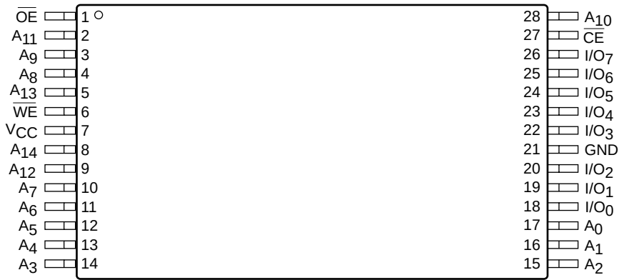
TSOP Top View (8mm X 13.4mm) (H)
