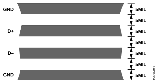
Figure 22. Typical Arrangement of Signal Tracks
